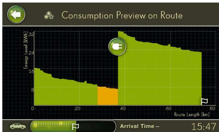
Figure 14: OBU displaying energy consumption preview on Route (Source: ELVIRE Delivery D2200 M15)
